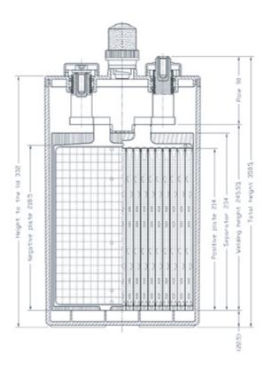
During assembling of OPzS blocks we need the bolted connection only between the end poles. All other poles of a block are also guided through the lid, providing sliding of the pole through the lid.
